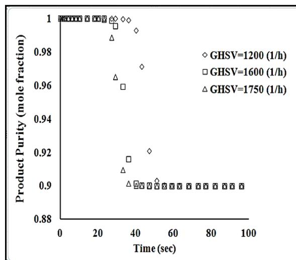
Figure 1. Breakthrough curve for the purification of  $H_2$  using 5A molecular sieve, at 40 atm and 40°C
