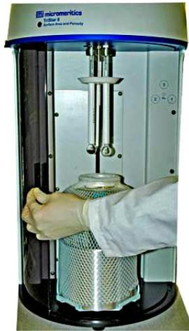
Figure 3. The sample compartment
