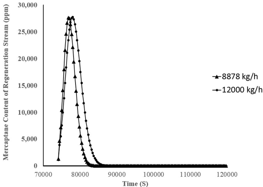
Figure 3 Mole fraction of mercaptans versus time in the gas stream during regeneration
