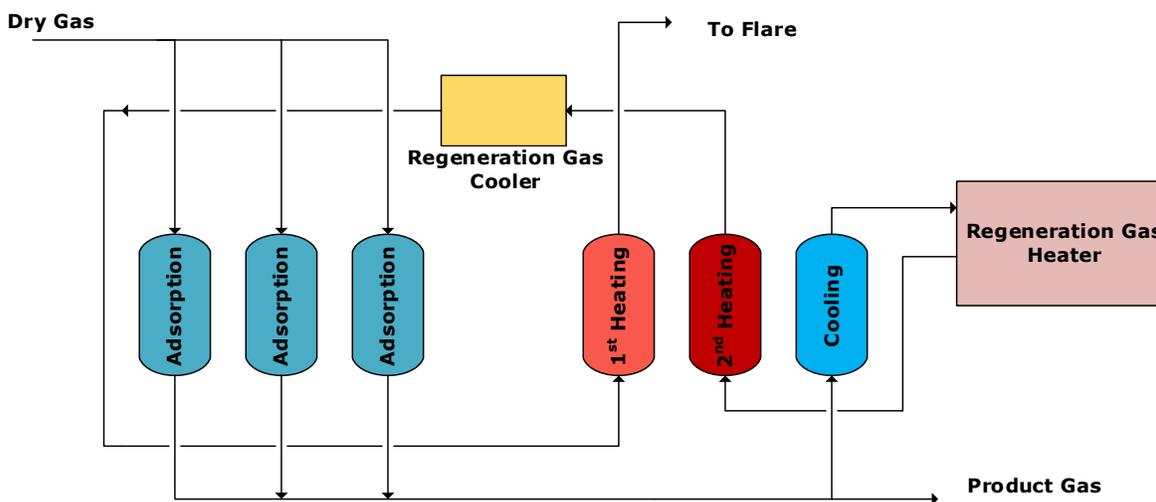
Figure 1. Schematic diagram of mercaptans removal unit (MRU)
