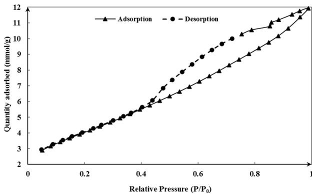
Figure 6. Adsorption and desorption isotherm of N<sub>2</sub> on HYAA300 (P<sub>0</sub> refers to standard pressure, 101.325 kPa).
