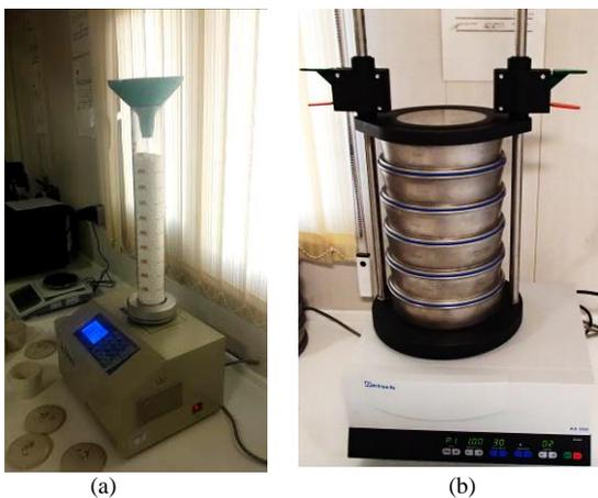
Figure 3. Tapped bulk density device (a) and sieve analysis device (b).
