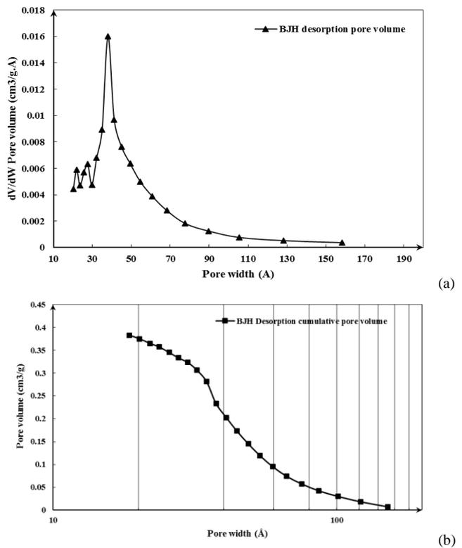
Figure 8. Pore size distribution of HYAA300 (desorption).
