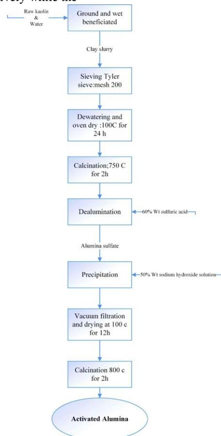
Figure 1. Flow chart for the synthesis of activated alumina from a type of binder.
