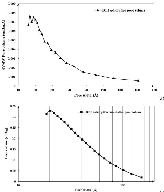
Figure 7. Pore size distribution of HYAA300 (adsorption).
